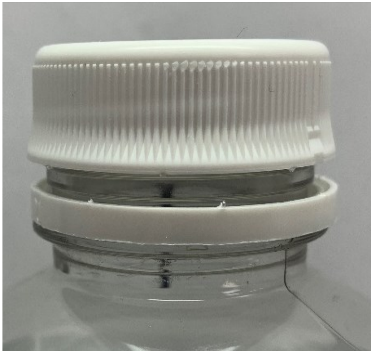
Figure 9: Closure rotated until all TE band bridges are broken.
