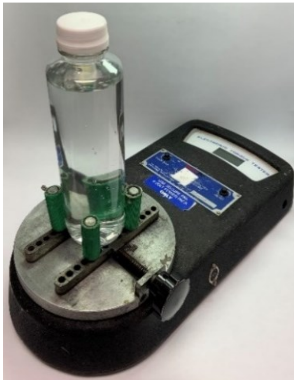
Figure 8: Proper hand removal torque setup
