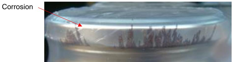
Figure 3: Filiform corrosion example
