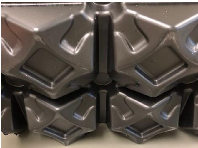
Figure 3: Proper tray design for even weight distribution
