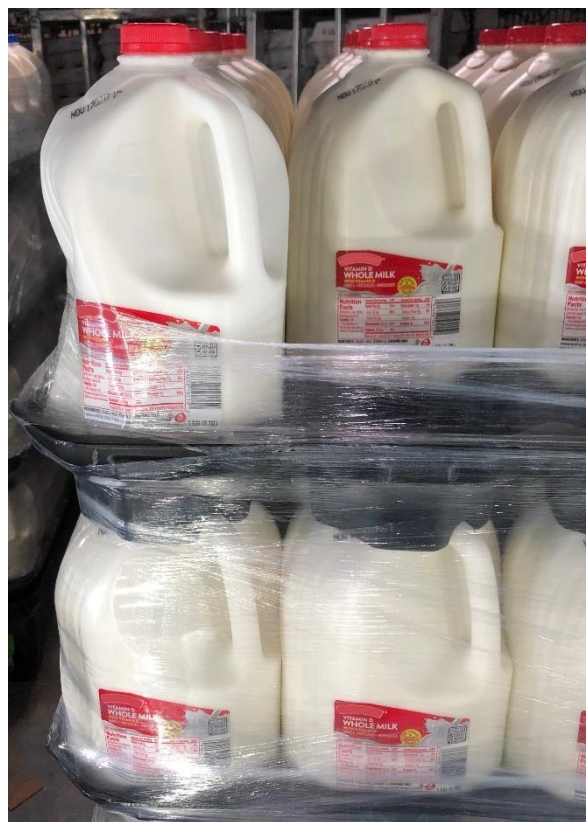
Figure 4: Example of excessive shrink wrap tension
