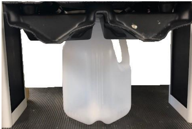
Figure 2: Proper load application to the bottle shoulder
