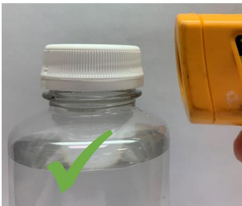
Figure 13: Correct cap shell temperature reading.
