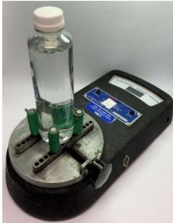
*Figure 8: Proper hand removal torque setup*
