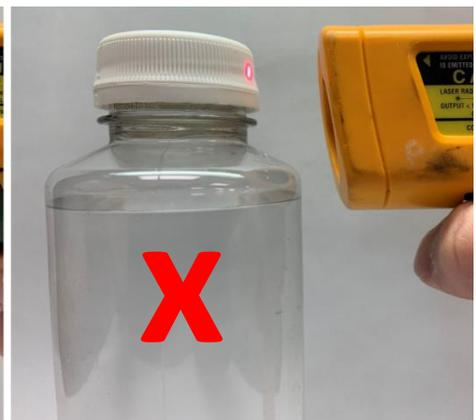
Figure 15: Incorrect low cap shell temperature reading.
