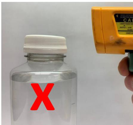
Figure 14: Incorrect high cap shell temperature reading.
