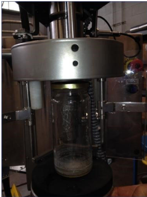
Figure 3-1: Manual Adjustment of Lift Plate
