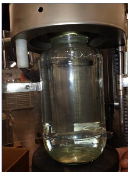
Figure 3-3: Plastic Pin to Adjust Head Height
